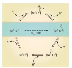
A minimal hydrogenase mechanism. The catalytic cycle shown for the core of [NiFe]hydrogenases is based on the constraints that only protons and electrons can enter or leave the active site, and do so singly. The reaction and species highlighted in blue is the equivalent chemical transformation reported by Ogo *et al.*; OMe<sup>-</sup> is the methoxide ion.
